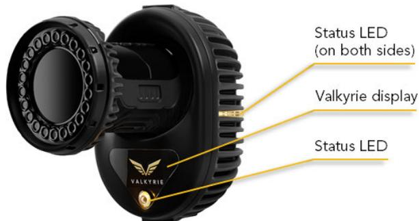
When the camera is communicating with Vicon application software, the status LEDs turn blue and the Valkyrie display shows the camera number.
